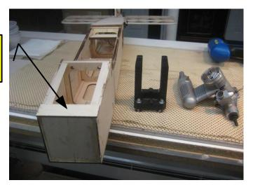
\*Cut, fit and glue in place 1/4"x1/4" balsa sticks to form the top truss construction reinforcements between formers #6 and #5 and then between formers #5 and #4.
