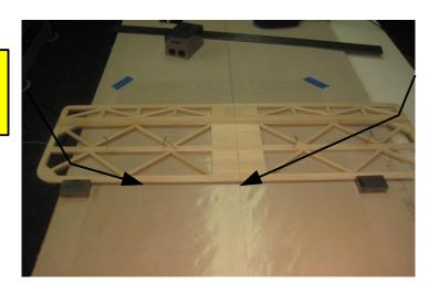
Line up stab center line to work surface center line
