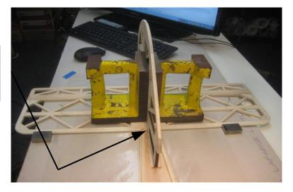
\*NOTE: The fuselage formers have locating tabs that will position them in the proper location on the bottom panel and both side panels. The bottom panel and the side panels will have slots to accept the former tabs. This locating method will also add strength to the plane.
