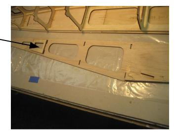
\*Cut, fit 1/4"x1/4" balsa stick along the top edge of the fuselage sides from the front surface of former #4 to the rear end of the fuselage sides. Bevel the inside surface of the balsa stick that is against the rudder surface. Remove 1/4" at the rear end to zero stock removal 2-1/2" forward from the rear edge. Glue in place.
