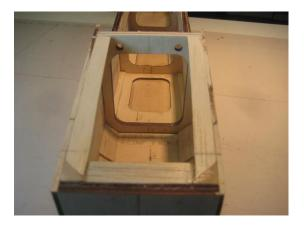
\*position and glue in place the laser cut 1/8" plywood hatch front.
