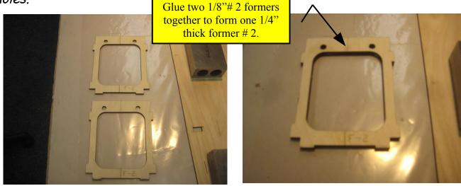
\*Position and hold in place fuselage former #2 in its corresponding location on the fuselage bottom using the tabs and slots for location. Make sure the former is held 90 degrees to the fuselage bottom and centered on the center line. Glue in place.
