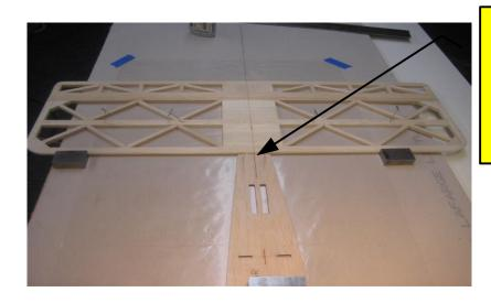
Bump fuselage panel to front edge of horizontal stab, lining up the center lines and line up the center line on the front of the fuselage panel to the center line on the work Surface. Glue in place.
