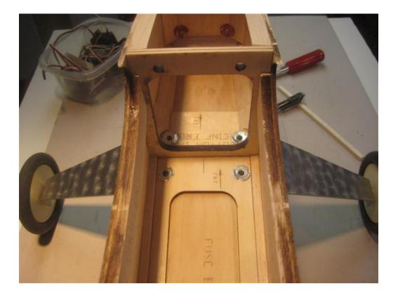
This is the point where the main wing is positioned and attached to the fuselage.
