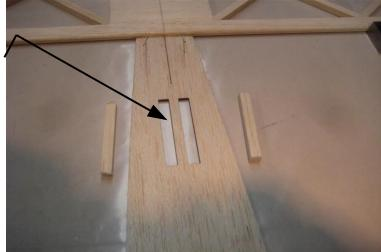
Glue locating blocks in the slots of the bottom Fuselage panel.. \*Fit and position the vertical fin on the center line of the horizontal stabilizer with the offset in the vert. fin against the front edge of the horizontal stab and between the two balsa locating blocks glued in the slots of the bottom fuselage panel assembly. Glue the vertical fin in position, making sure the fin is perfectly 90 degrees to the horizontal stabilizer. Block in place while glue dries.
