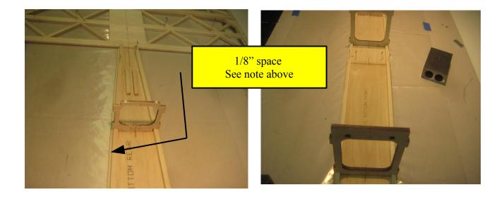
\*Position the laser cut plywood bottom I/S reinforcement with the arrow facing forward and on top of the fuselage bottom between formers #4 and #2 and between the 1/4"x1/4" balsa sticks. Glue in place.
