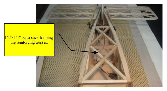
\*Cut, fit and glue in place 1/4"x1/4" balsa sticks to reinforce the wing mounting panel.
