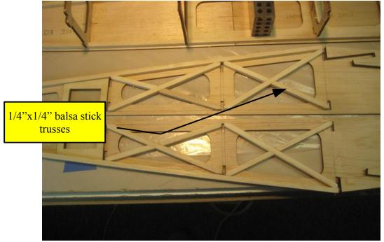
\*Cut off the bottom 1/4"x1/4" balsa sticks flush with the front surface of former #2.
