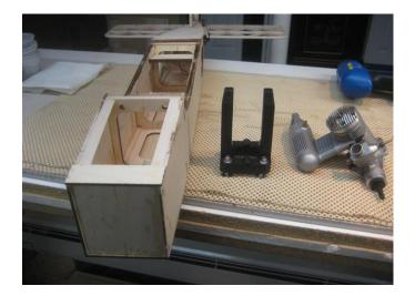
\*Position the fire wall in place using the tabs and slots for location. Make sure you glue the fuselage sides to the fuselage bottom. Glue the forward firewall against the locating firewall. Epoxy in place.
