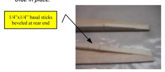
\*Cut, fit and glue in place 1/4"x1/4" balsa sticks to form truss construction reinforcements between formers #6 and #5 and then between formers #5 and #4.
