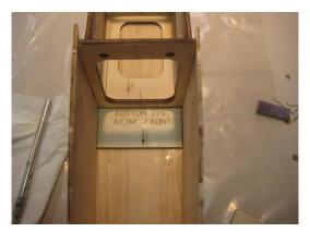
\*Cut and fit supplied balsa triangle sticks to all the corner joints in the front area between former # 2 and the firewall.
